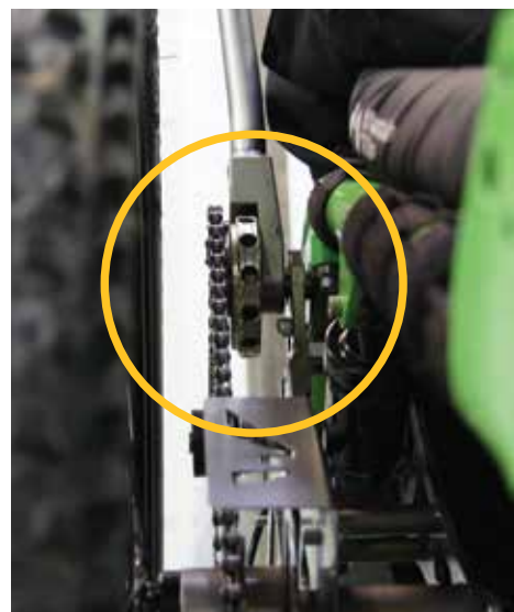
The Stieber overrunning clutch offers far more in terms of reliable performance and is now specified as standard on all Mountain Trikes.
