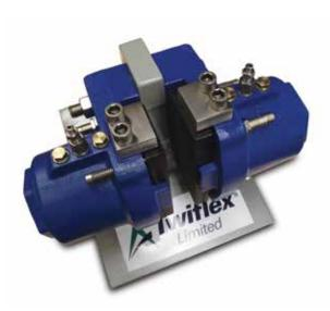
The VBS will be introduced as the smallest brake in the Twiflex modular range – a range which continues to grow – with a braking force of 1.4 to 11 kN. The brake is designed to deliver 2 million cycles at 2 mm air gap. It features a stainless steel piston, cover plate and fittings and optional ISO 12944-5:2007 C5 paint specification.
